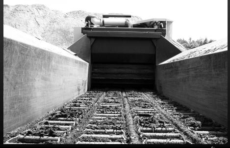
Carrier aggregate used to keep Shingles from agglomerating and allow to flow through cold feed bin
